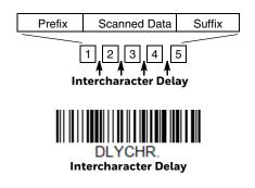
To remove this delay, scan the **Intercharacter Delay** barcode, then set the number of delays to 0. Scan the **Save** barcode from the Programming Chart, beginning on page 311.
