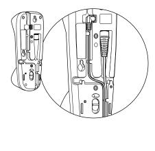
5. Replace with the new cable. Insert the connector into the opening and press firmly. The connector is keyed to go in only one way, and will click into place.
