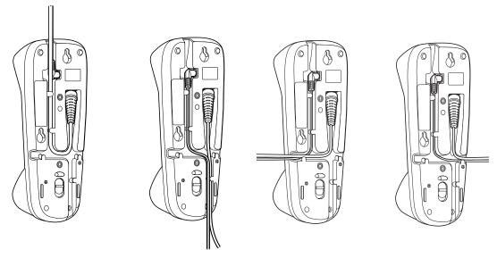
When mounted on a vertical surface, a locking system is used to secure the scanner when it is in the stand. When mounted on a horizontal surface, the locking mechanism should be set to unlocked (pushed down). When mounted on a vertical surface, the locking mechanism should be set to locked (pushed up).
