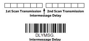
To remove this delay, scan the **Intermessage Delay** barcode, then set the number of delays to **0**. Scan the **Save** barcode from the Programming Chart, beginning on page 311.
